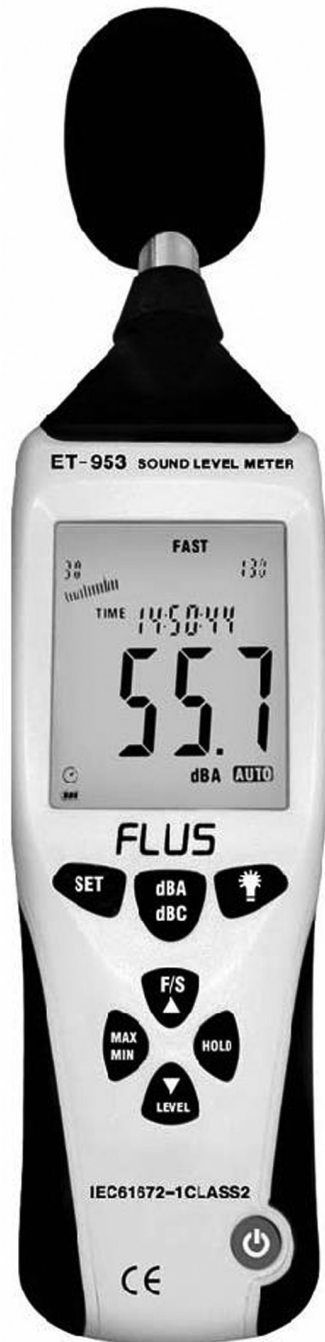
Figure 17.2 Sound level meter to measure noise levels.
